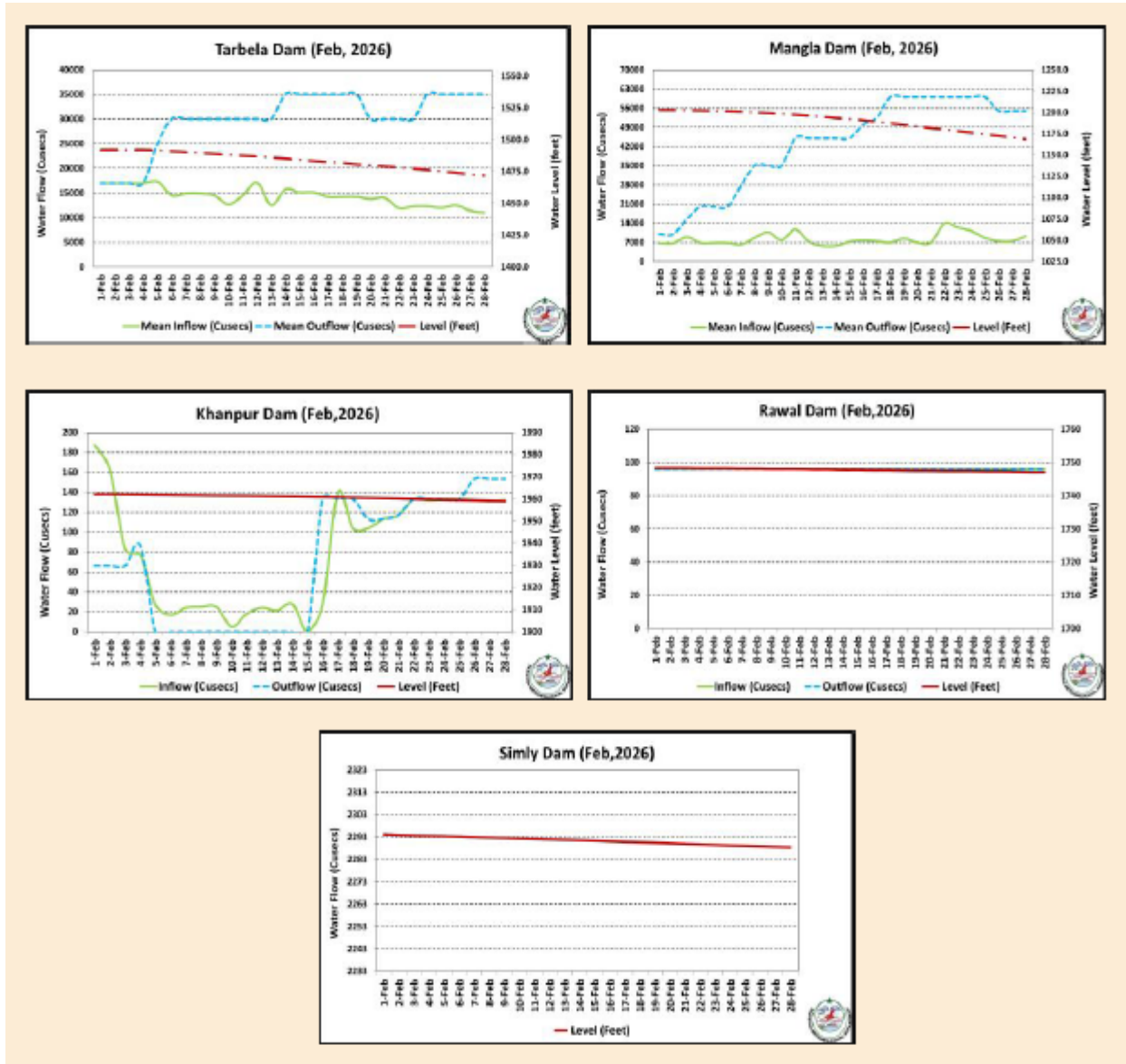
Water inflow, outflow and level of Rawal, Khanpur, Tarbela and Mangla Dams
